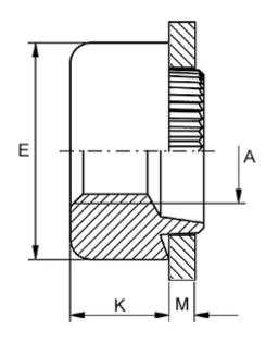
Female thread A = M2Height K = 3.0Outer diameter E = 8.0Plate thickness = 4.1 to 4.3
